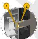
1 – Impeller without fixing nut.
