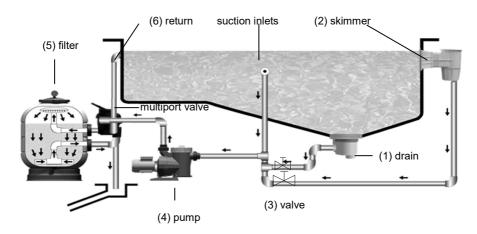
A suction is taken from the main drains (1) on the bottom of the pool and the skimmers (2) at the pool surface and fed via separate pipe work with their corresponding valves (3), through the pump (4) to the sand filter (5).
