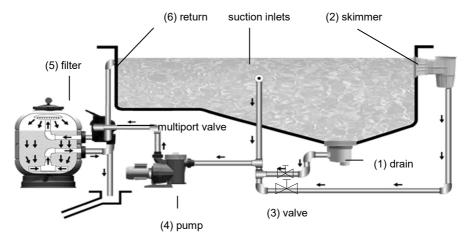
A suction is taken from the main drains (1) on the bottom of the pool and the skimmers (2) at the pool surface and fed via separate pipe work with their corresponding valves (3), through the pump (4) to the sand filter (5). After filtration, the water is returned to the pool via return inlets (6), which are installed on the opposite side of the pool to the skimmers and main drains.
