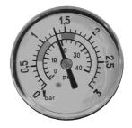
1,3 kg/cm² - 18,5 PSI: This pressure indicates that it is necessary to "BACKWASH"
